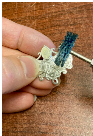
Protect the Opals when using a rotary tool by covering it with masking tape.
