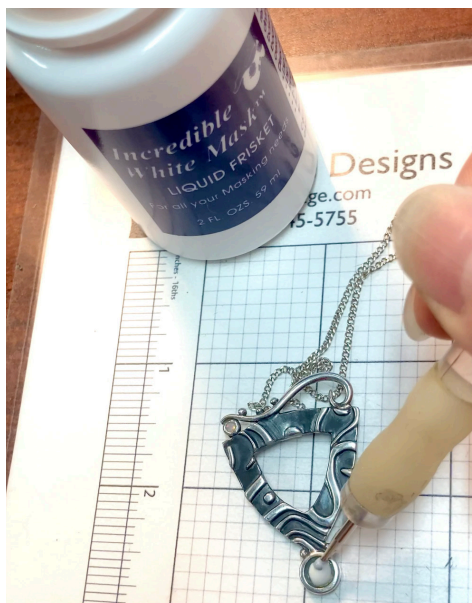
Grafix® Incredible White Mask Liquid Frisket is used to protect the Opals in the tumbler and to resist LOS from getting on the metal behind the stone.
