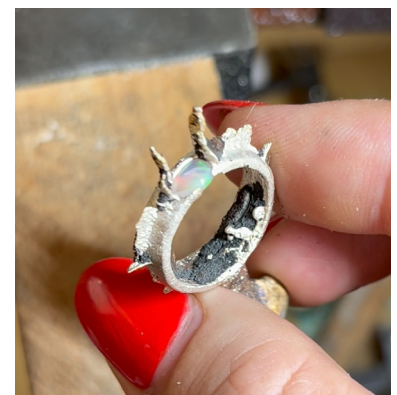
Remove the Cooled Metal Casting
