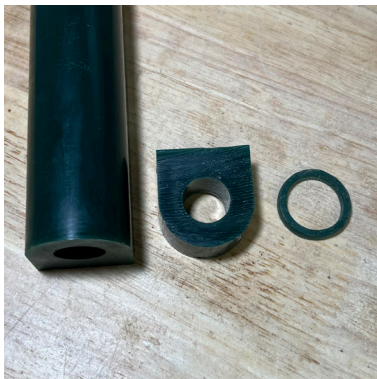
The Jeweler's Wax used to Carve the Ring Design
