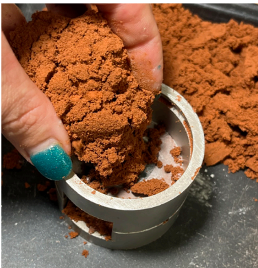
Add the Female and Fill the Flask with Sand
