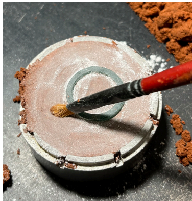
Wax Model is Pressed Halfway into the Sand and Baby Powder is Brushed Over the Top
