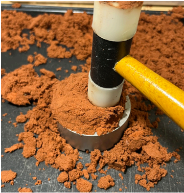
Sand packed into the Male Side of the Flask
