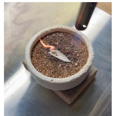
Torch Firing on Vermiculite
