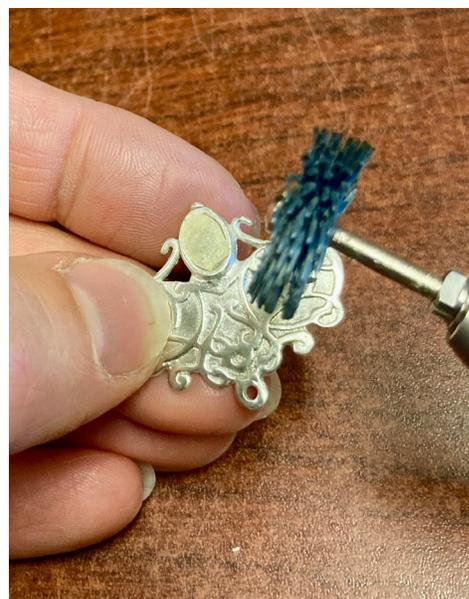
*Protect the Opals when using a rotary tool by covering it with masking tape.*
